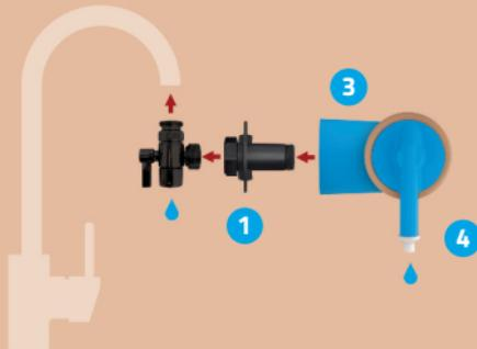
All components except the Ujeta water filter are not included in the scope of delivery
